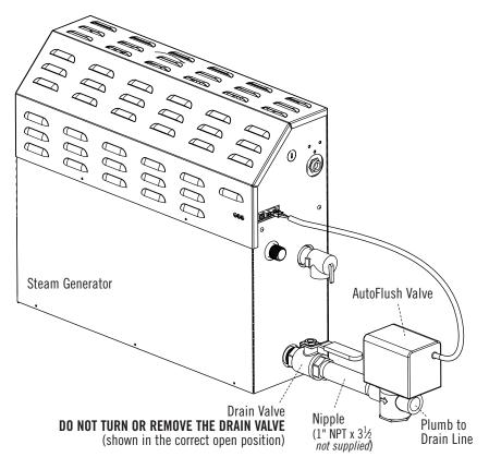
Our exclusive AutoFlush automatically and electronically drains the system, providing CleanSteam... Every Time® and introduces fresh water.
