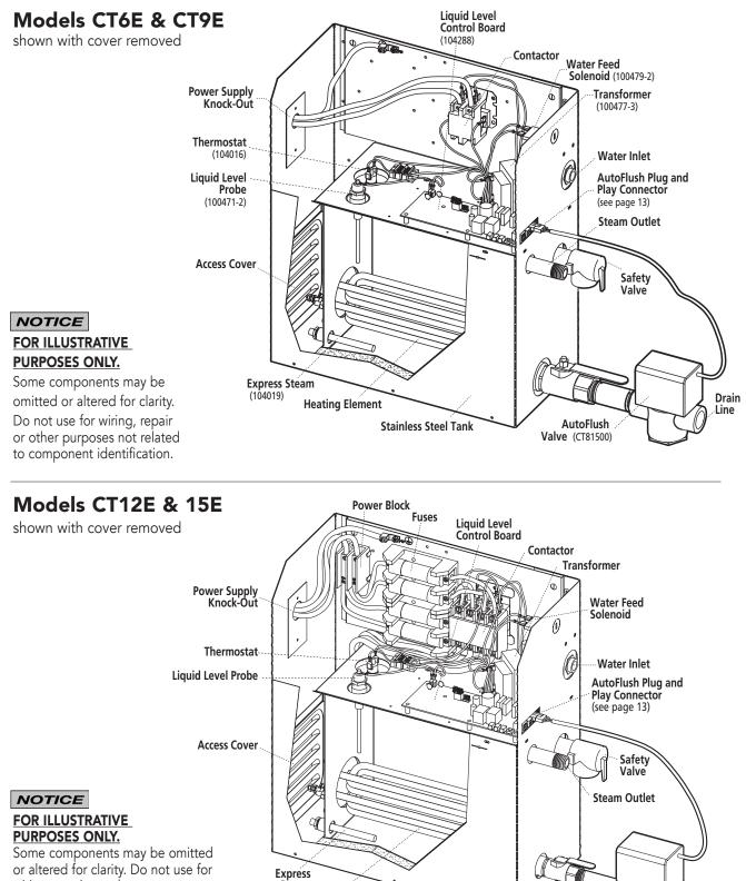
or altered for clarity. Do not use for wiring, repair or other purposes not related to component identification.
