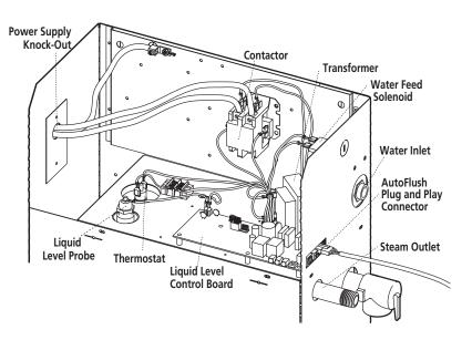
main voltage on the load side of the contactor when it is engaged.
