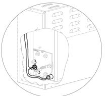
All CT models have Express Steam standard. Express Steam is equipped with a low power heating element and thermostat to keep the water in the tank warm enough to bring up steam quicker. All Express Steam components and wiring are installed at the factory. No additional wiring or plumbing is required by installers.
