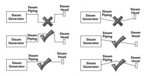
4. Flush inlet water line thoroughly before making connection to unit. A warning Failure to pitch the steam piping as required for condensate to drain, may cause condensate to block the flow of steam. Blocking the steam flow may cause steam pressure to discharge boiling water through the steamhead, resulting in a scalding hazard. Blocking the flow of steam may cause steam to discharge through the safety valve, resulting in a scalding hazard.
