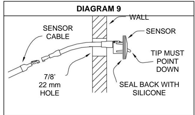
Run a light bead of silicone around the back surface of the sensor and slide it into the wall with the metal sensor tube pointed down. Tape the sensor to the wall until the silicone has set-up.
