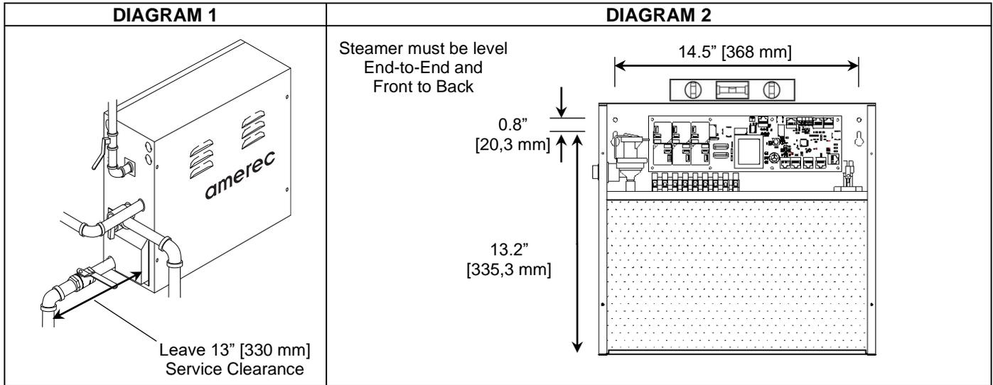
The AMEREC steam generator can be hung on a wall or sit on its base. The best mounting location will satisfy all or most of the following:
