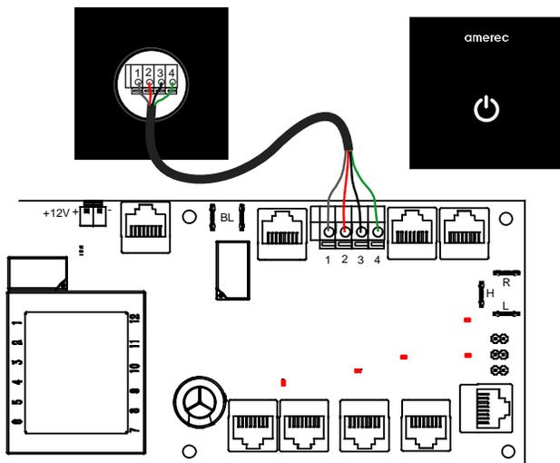
Use a small screwdriver to push the terminal block tabs when installing or removing wires.
