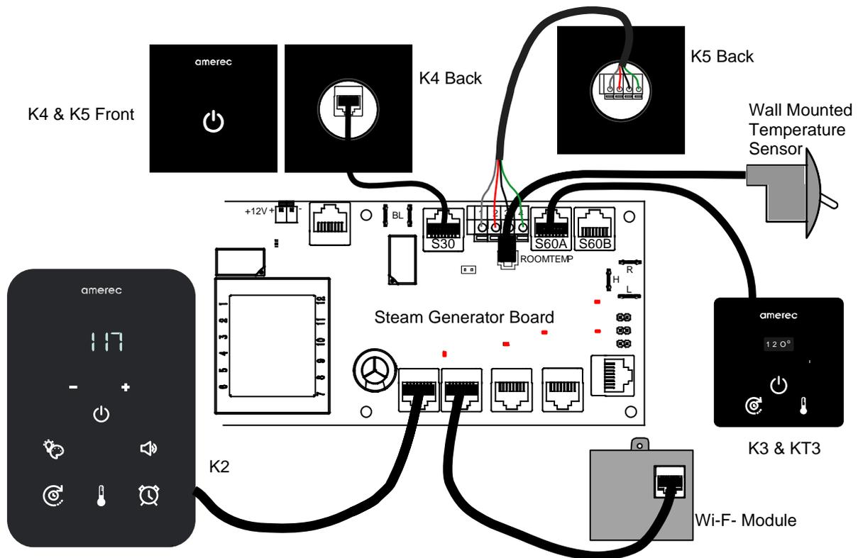
**Note:** The K2 and K3 controls provide bath temperature and run time control and they require a temperature sensor. The K4 is an on/off control used to start and stop the bath but they do not have temperature control. When using only a K4, turn the bath on when it is too cool and, if the bath becomes too hot, turn the bath off.
