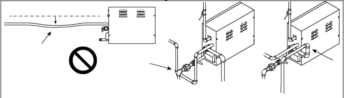
**Note:** See Diagram 6 for a typical installation. Additional steam heads may be added to any installation to reduce steam noise or to provide more steam dispersion around a large room. *For large AK14 steamers, we recommend using 2 steam heads to reduce the noise level while steaming.*
