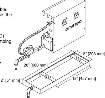
DO NOT drain the drip pan into the steam bath.
