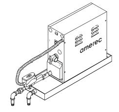
DO NOT connect the steamer and drip pan drains together!
