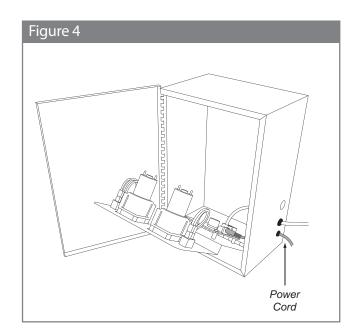
6. Plug the power cord (supplied) into the TSA AromaSense Module's circuit board (shown in Figure4 and Figure 8) and to an outlet. Make sure the pump rollers spin (6) when the switches are pressed on the TSA AromaSense Module. If the pump does not spin check that the power supply is securely plugged into the pump control circuit board located behind the pump panel.
