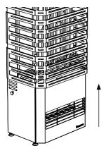
Remove the output grille by holding it slightly tilted and pulling it downwards.
