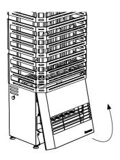
Pull from under the output grille edge outwards.
