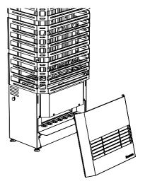
Place the salt in the sockets. To simplify the operation, the salt tray can be removed.
