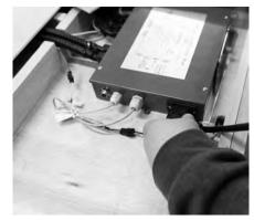
**4**. Replace the power supply cover screws.
