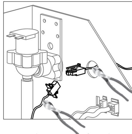
1. Remove the connector from the "C" location in the jacket. Cut off the connector where shown and strip back the wires approx 0.375"
