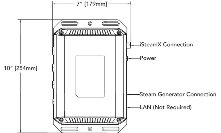
The iSteam controls are designed to be installed inside or outside the steam room but is primarily installed inside the steam room. If the control is installed inside the steam room the control must be located:
