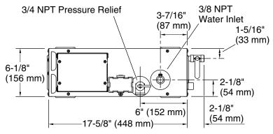
Minimum required access panel is 24" (610 mm) L x 15" (381 mm) H.
