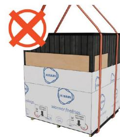
Do not lift the sauna with slings set from side to side. Doing so, will damage the sauna.
