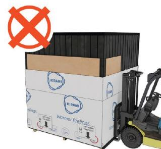
Do not drive the forklift from the side. Doing so, will damage the sauna.
