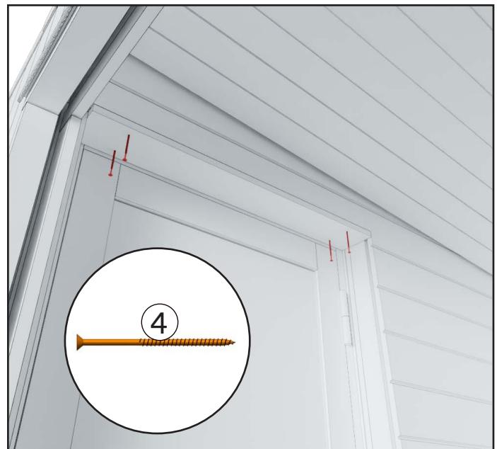
2. Place a short cover board at the top of the doorway so that the front edge of the board is at the same level as the inner wall of the module.
